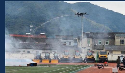
The C.FC100XF is a high-end tethered firefighting drone system designed for long-duration aerial operations. With 30 kW onboard power, high-strength tether, and versatile firefighting payloads, it provides stable, precise, and safe support for urban, forest, and industrial emergency response.
