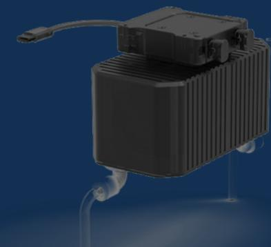
The C.GS100P is a drone-mounted gas sampling device specifically developed for environmental gas collection. It features a professional gas pump for pollution-free extraction into sampling bags, an intelligent bag cleaning system to prevent cross-contamination, and a smart pressure sensor that automatically stops sampling when the bag is full.
